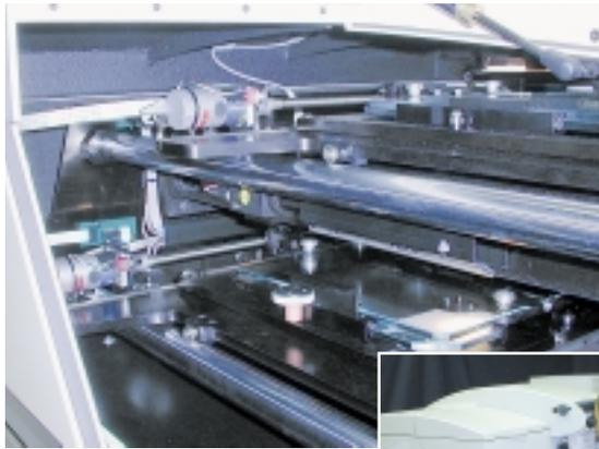
The ORTHO System 2 is unique in that the scanning and orthophoto rectification is done in a single step. Only the final ortho image is ever stored! There is no need to scan and store all the intermediate image files that a softcopy system would require.
